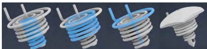
Fig. 1 Multilayer design boosts magnetic flux density, while custom 3D-printed resin components ensure coil stability.
