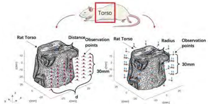
Fig. 1 The planar sensor array and proposed cylindrical sensor array
