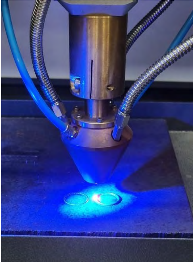
"3D printing of potential TMS coil magnetic material using directed energy deposition"
