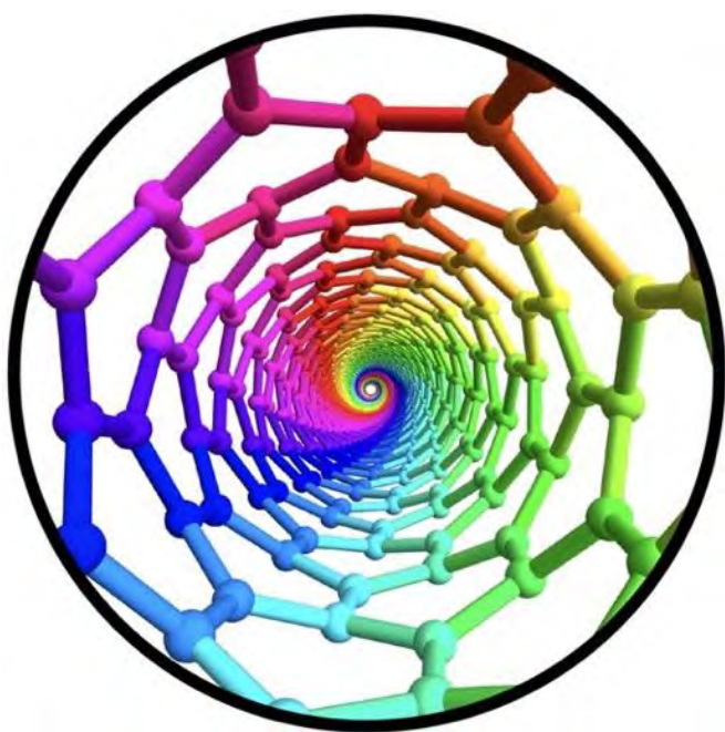
Fig. 2 View into a chiral carbon nanotube. The color is assigned based on the underlying graphene layer and visualizes the chirality of the tube. From [6].
